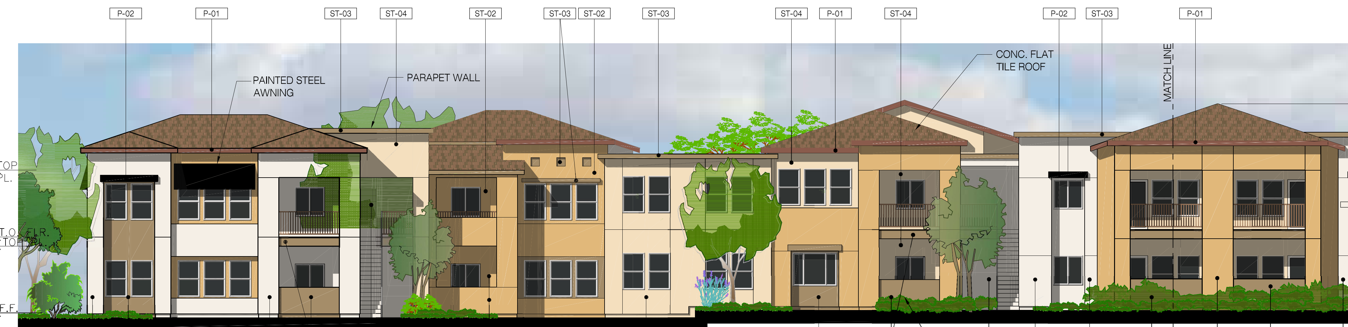
PARTIAL COURTYARD ELEVATION
